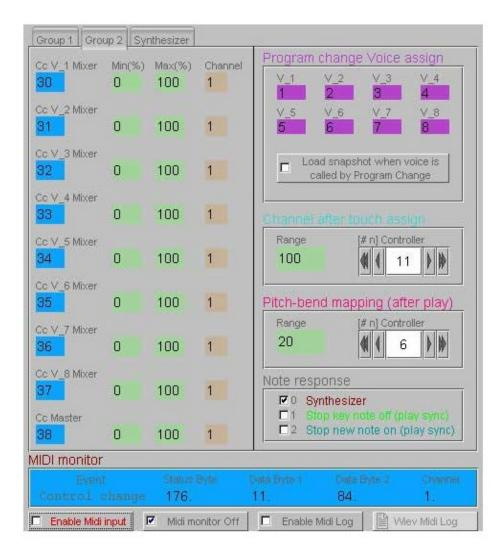
The group manages two controls assigned to the mixer using the control change and program changes are being made to select items; possibly can switch the voice call load on the snapshot.
