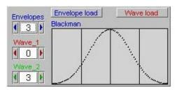
The default density using an envelope for grains of type Hanning. There are 11 types of windows. The slope of attack and decay of the prototype can be modified by the controls [# 2] Attack [# 3] Decay and displays the result on the appropriate scope.
