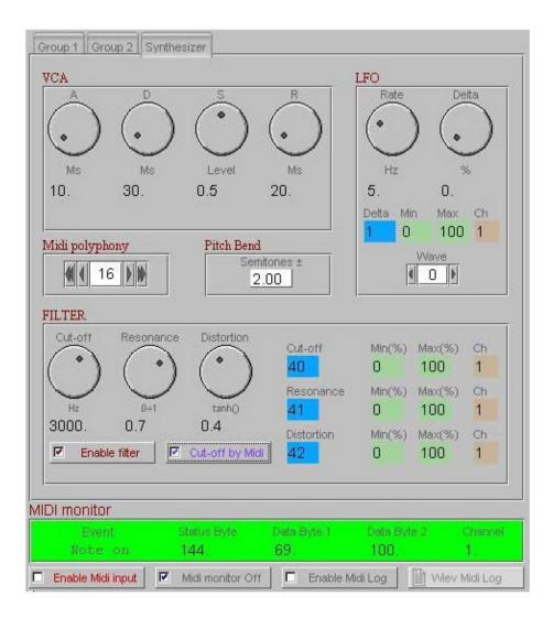
The Sinthesizer has a classic ADSR envelope generator (Attack-Decay-Sustain-Release) You reported the event. Weather explained in R (release) extends the "notes" after the note-off message (note-off sensor and release time extender).
